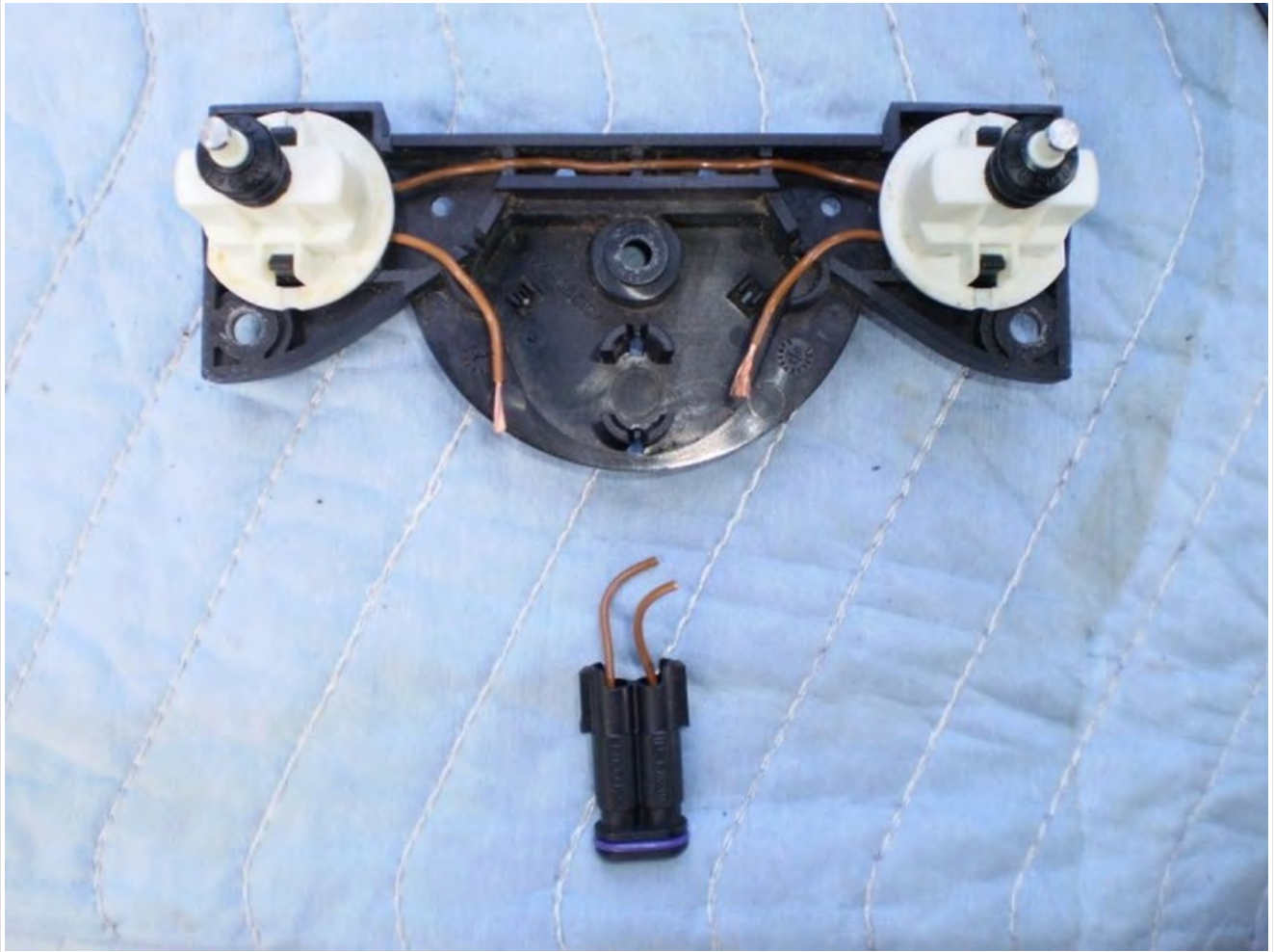
39. Splice, solder, and heat shrink the longer end of the trailer connector to the SVS wires and run them through the SVS cover plate.
