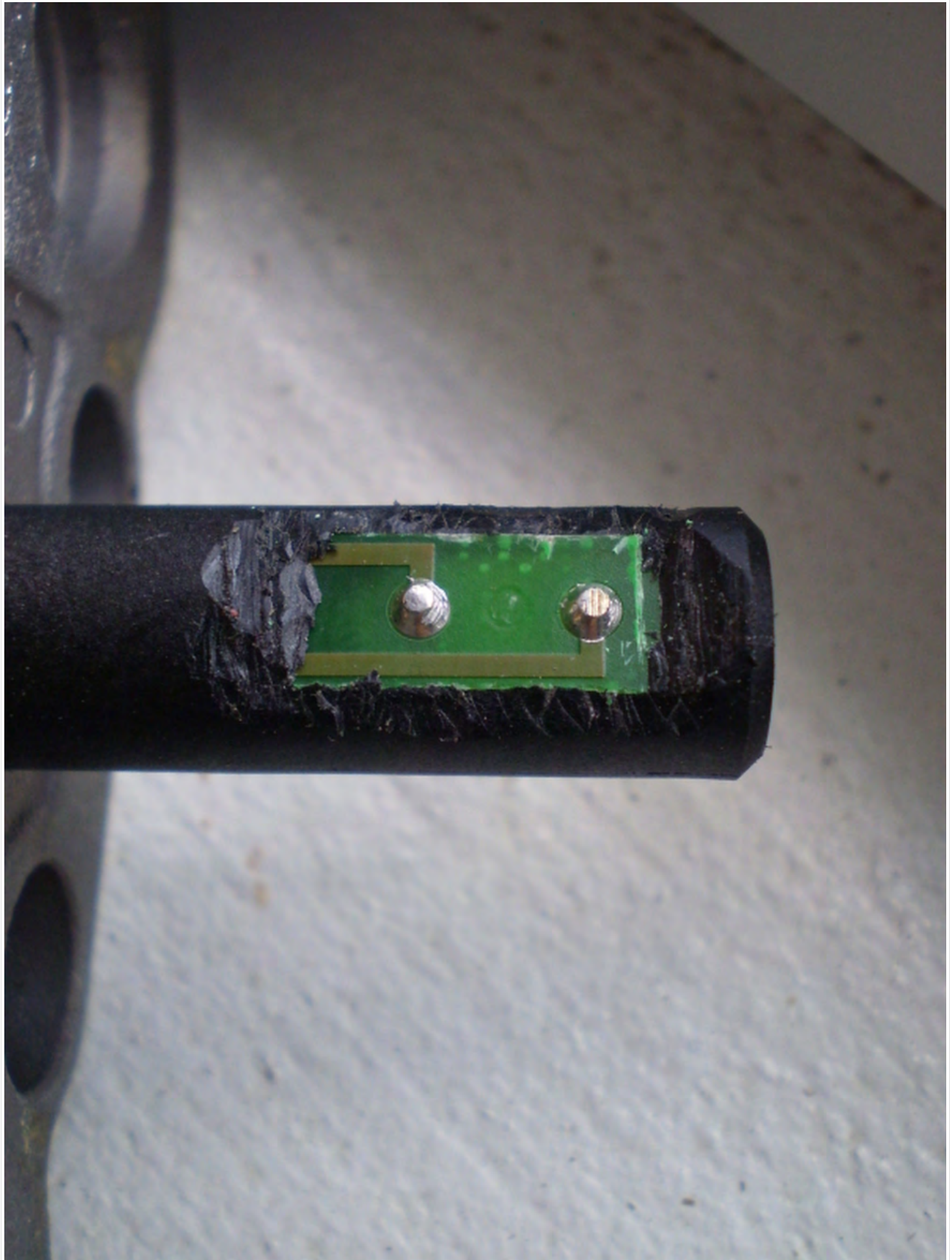
35. Upon inspection of my circuit board and that of the spare's, I found it very hard to tell if the soldered joints were bad. Both pins remained on the circuit board when I removed the SVS plug but I could tell they weren't 100% solid. I re-soldered the pins on the spare unit. Be careful as the pins may fall out. while soldering. One did fall out but I was able to reinsert it with pliers and re-soldered it. I re-tested the SVS on all three positions and passed.
