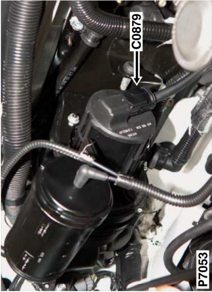
Description: Pump-Air injection Location: Rear RH side of engine compartment
