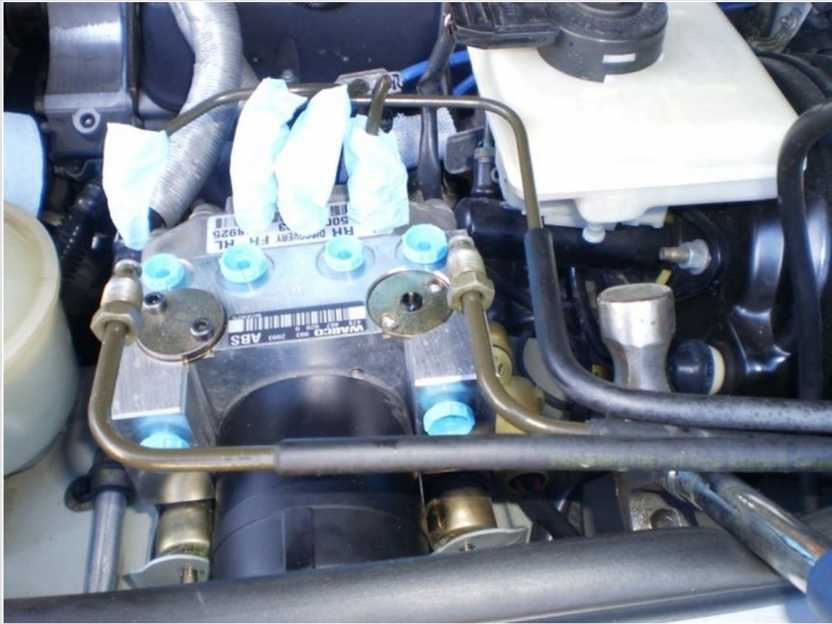
12. Lift the front of the modulator and remove the front rubber mount.
