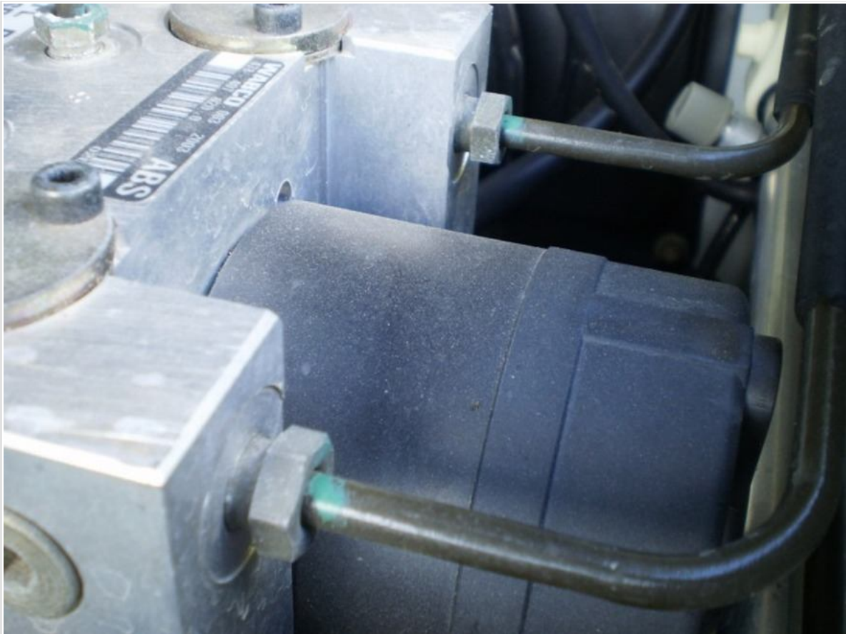
8. Once all 6 brake lines are broken loose, remove the 3 nuts securing the modulator on to its mounting bracket using a 10mm wrench.
