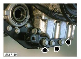
**21.** Remove 3 bolts securing lower engine steady bracket to sump and remove bracket.
