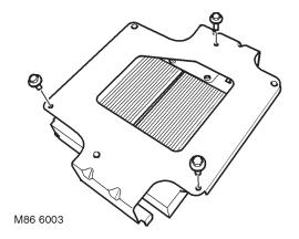
4. Remove 3 bolts securing power amplifier to cradle and remove power amplifier.
