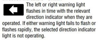
**NOTE:** If the hazard warning lights are operated, both direction indicator warning lights will flash together.
