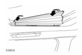
4. Loosen the 4 roof opening panel Torx screws.
