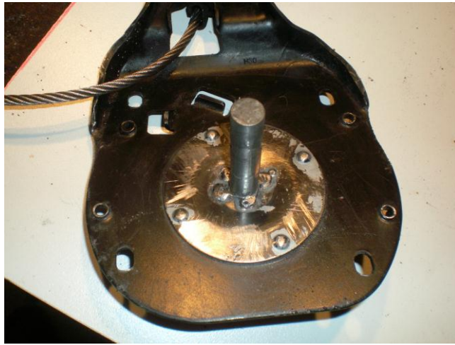
Figure 6 Shaft and Lower Clutch Plate Installed
