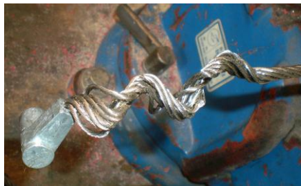
Figure 1 My Winch Cable Kinked
