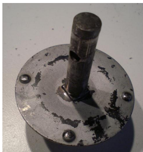
Figure 5 Repaired Shaft and Clutch Plate before installing in the Casing
