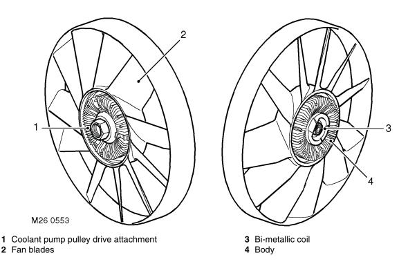
The viscous fan provides a means of controlling the speed of the fan relative to the operating temperature of the engine. The fan rotation draws air through the radiator, reducing engine coolant temperatures when the vehicle is stationary or moving slowly.
