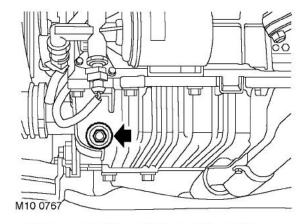
Place a suitable container under engine sump drain plug, remove plug and discard sealing washer. Allow oil to drain.
