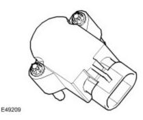
The high/low position sensor converts the pivotal movement of the high/low fork into a PWM signal on the input. The PWM signal of the position sensor differs between high range and low range. The control module checks this signal and informs the driver, via the instrument cluster and the range change selection switch LED's, if a range change is in progress or has been completed.
