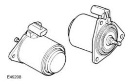
The solenoid switches the power flow on the actuation system between high/low range change mode and clutch control mode. When the solenoid is energized, the solenoid pin deploys and activates the clutch control mode. When the solenoid is de-energized, the internal spring rejects the solenoid pin and activates the high/low range change mode.
