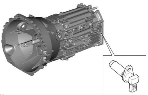
The output shaft speed sensor is located at the rear of the transmission and measures the speed of the transmission output shaft.
