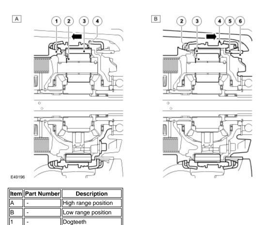
When high range is engaged, the shifting sleeve (4) connects to the differential carrier via dogteeth (1). The planetary ring gear (3), via the shifting sleeve, and the planetary pinion gears (5), via the planetary shafts, are also attached to the differential carrier. The planetary gear set rotates as one unit and therefore turns the differential side gear with a 1:1 ratio.
