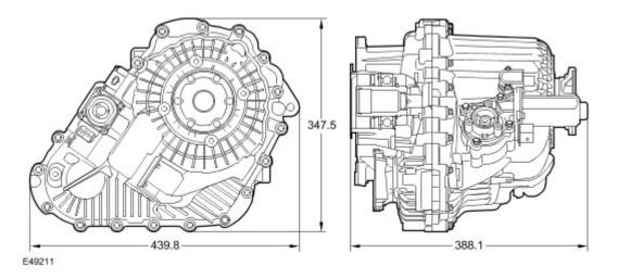
The transfer box weighs 40.30 kg without oil and 41.55 kg with oil. The unit requires 1500 ml  $\pm$  2% of oil from empty.
