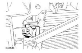
15 . Remove the A/C manifold bolt.
