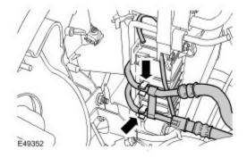
14. Remove the power steering fluid cooler line clip.
