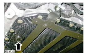
9 . Install the transmission fluid drain plug and tighten to  $9\ Nm$  (7 lb.ft).
