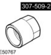
ZF Automatic transmission selector shaft seal remover 307-509-2 (LRT-44-033/2)
