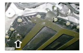
9. Install the transmission fluid drain plug and tighten to 9 Nm (7 lb.ft).
