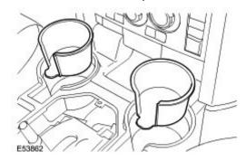
3 . Remove the floor console liner.
