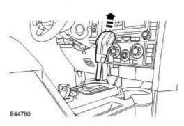
2. Release the ride and handling optimization switch assembly.
