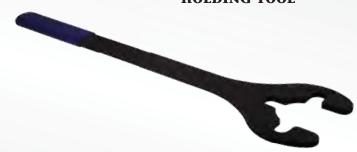
Allows the technician to hold the water pump pulley in place while loosening the radiator fan. Applicable to: Mercedes-Benz model 1998 & newer w/ 112 & 113 engines; Ford 2.8L, 2.9L & 4.0L V6 engines including 1991-2002 Explorer, F-Series w/ 4.9L in-line 6-cyl. engines w/ 36mm fan nut; & Land Rover Freelander w/ V6 engine.
