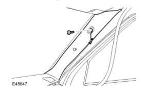
4. NOTE : Do not disassemble further if the component is removed for access only. Remove the screw retainer and clip from the A-pillar upper trim panel.
