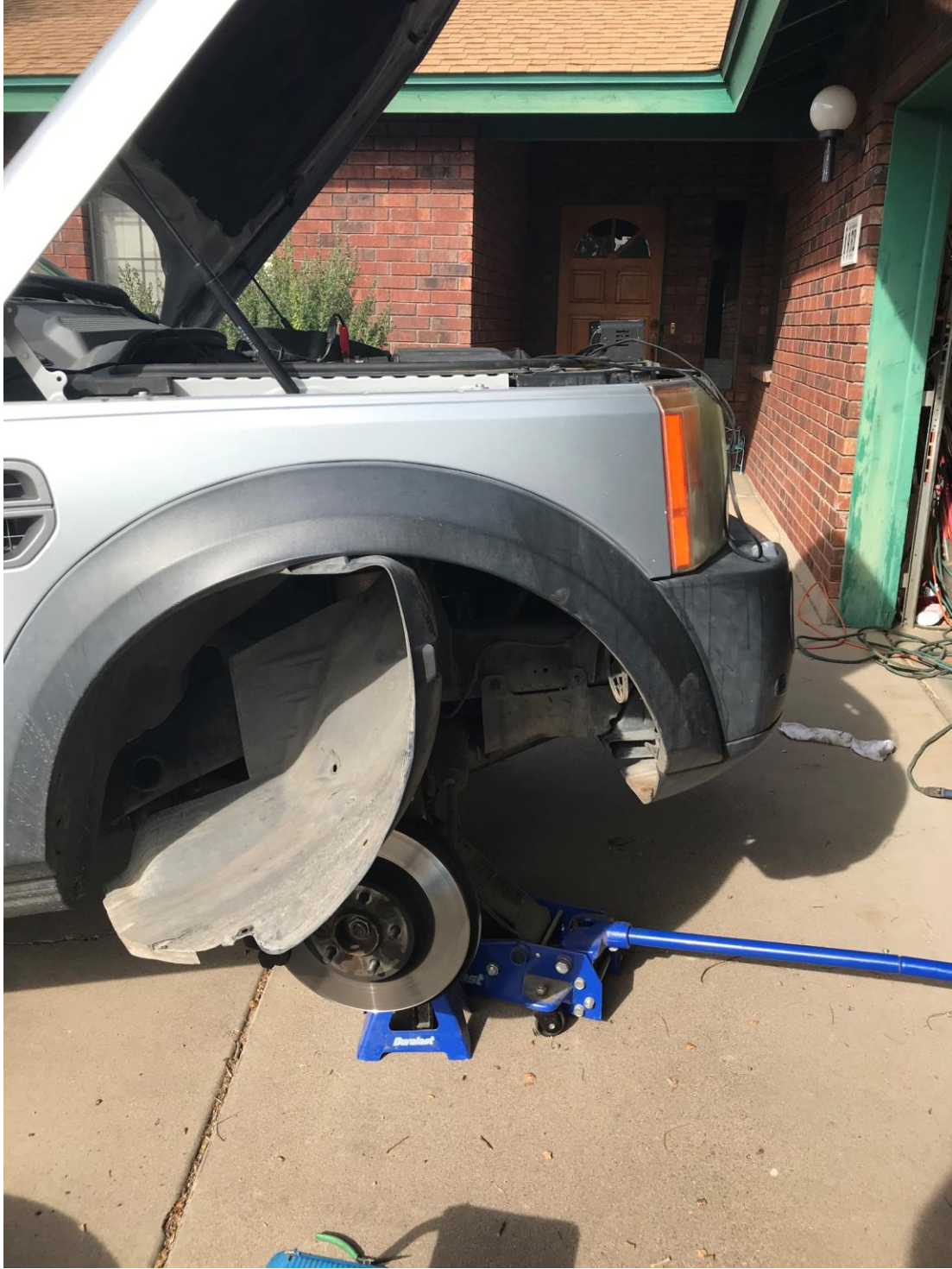
Jacked up the right front, peeled back the interior of the fender, to find the ground cable. From the battery ground, to ground the battery.
