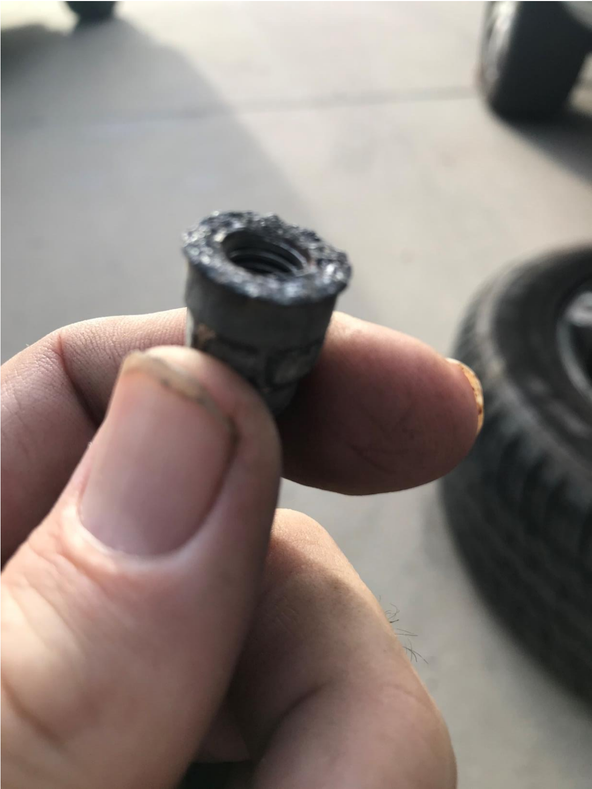
Removed the nut that holds the ground cable to the body. Obvious carbon build up and melting.
