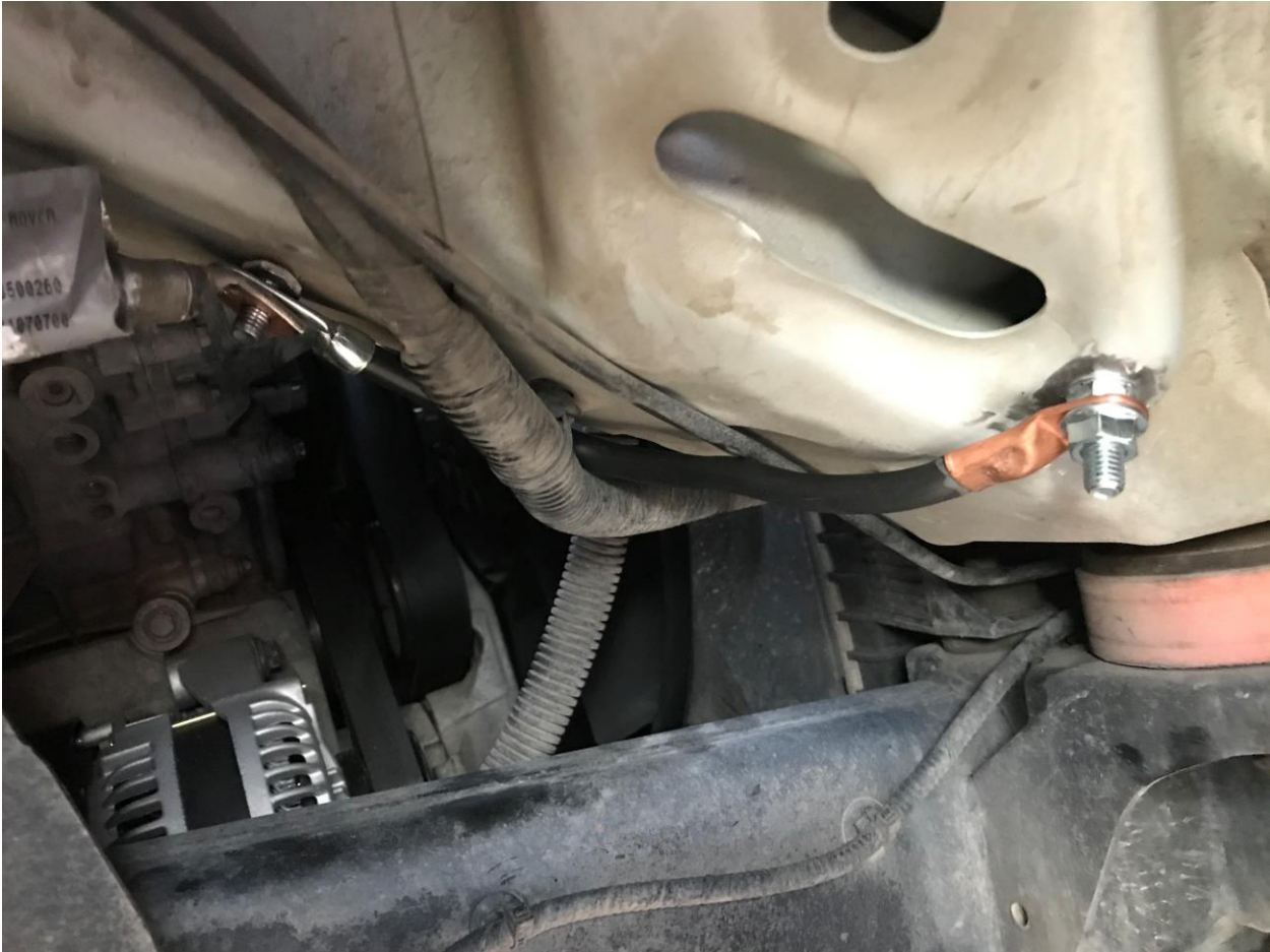
Added my own stud after cleaning away some paint.
