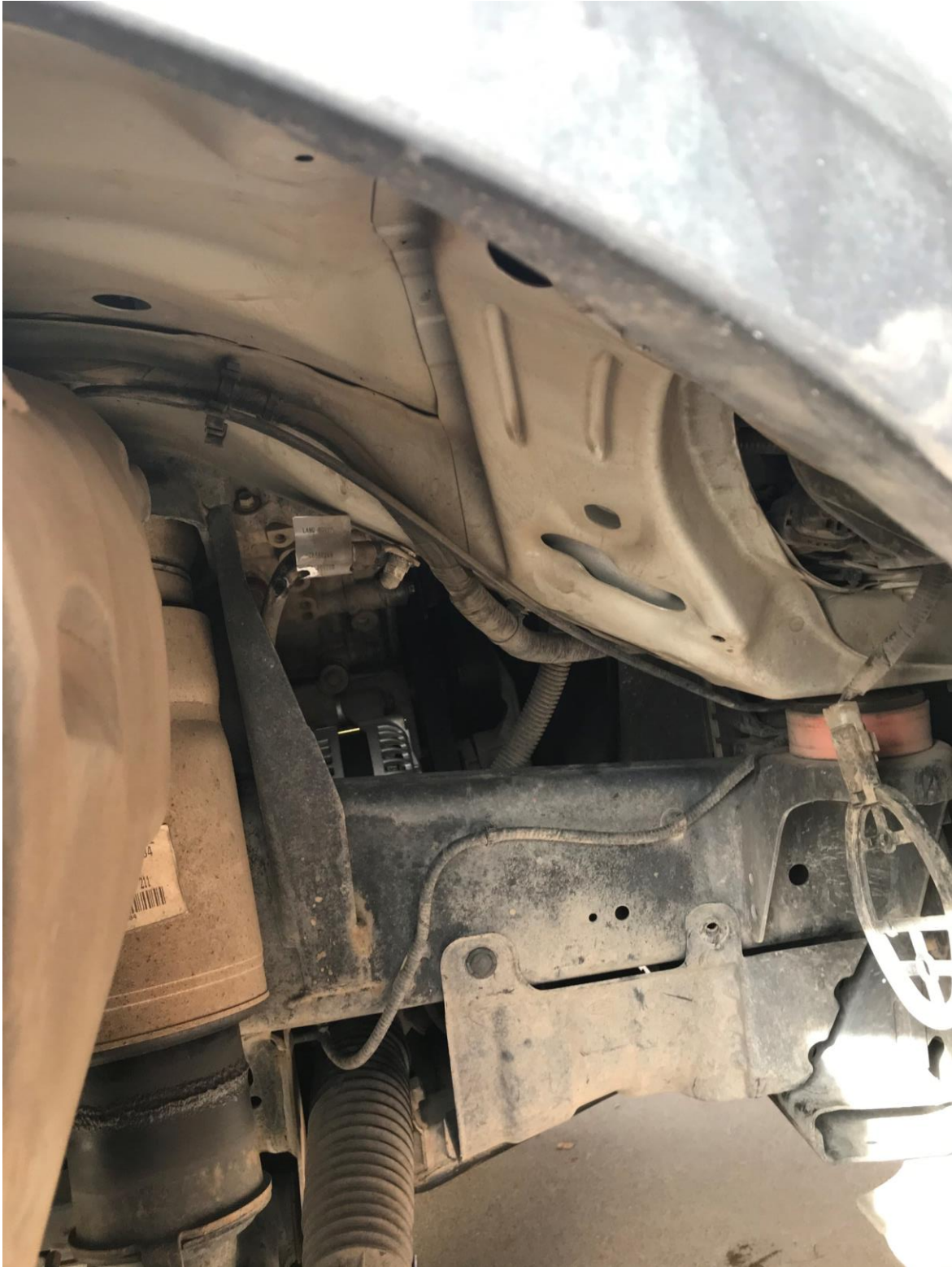
Found the ground cable on the body of the vehicle, inside the right front fender
