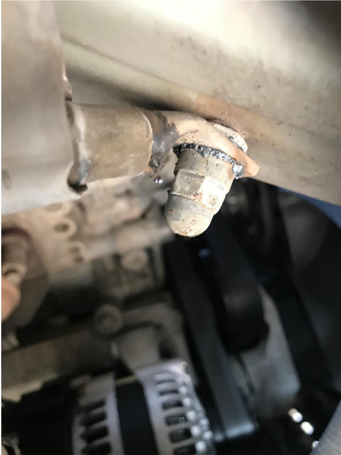
Close up of the battery ground cable, where it terminates on the body.
