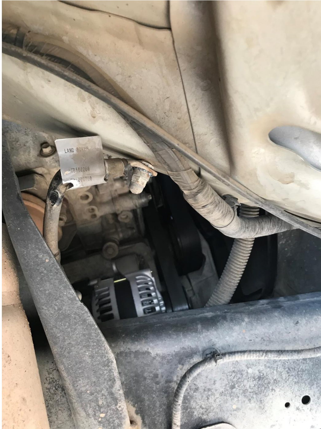
Inspecting the cable closely, you can see where it had been melting.
