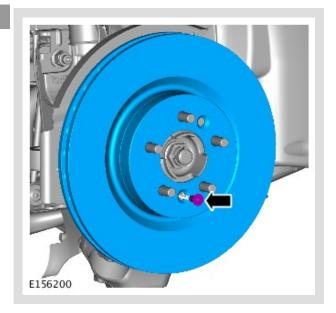
Remove the brake disc.
