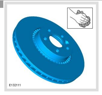
Clean the brake disc using brake cleaning fluid.
