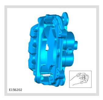
Clean the brake caliper housing and anchor plate using brake cleaning fluid.
