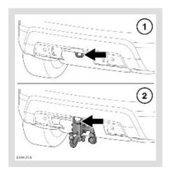
The vehicle towing eye is located in the following positions:
