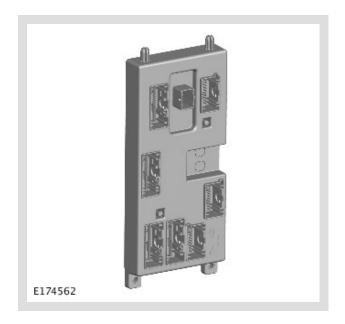
The Body Control Module/Gateway Module (BCM/GWM) assembly is attached to a bracket, which is bolted to the passenger side of the cross-car beam, behind the instrument panel.
