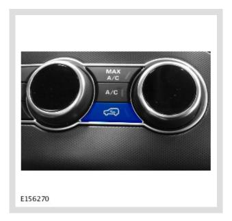
During this procedure, the ignition must remain in the ON position, and the A /C system must be in continuous recirculation mode with the fan speed set to minimum.
