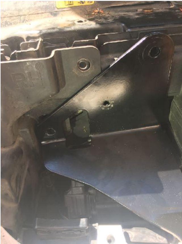
Image 5 showing horn attachment to bracket
