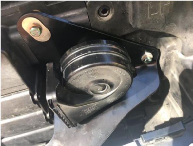
Image 5 showing horn attachment to bracket
