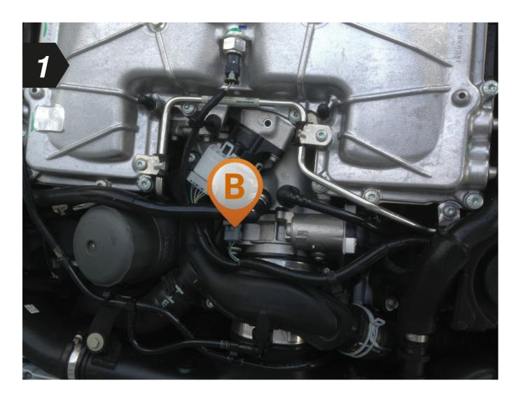
• To begin, locate the turbo boost pressure sensor in your engine bay.
