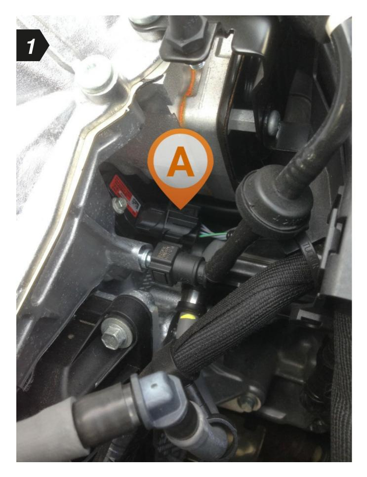
• To begin, locate the connection to the manifold absolute pressure sensor in your engine bay.
