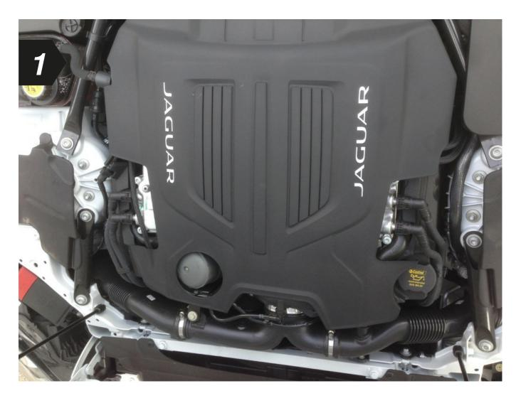
• Remove the engine cover and place it next to the car. You may have to jiggle the cover slightly to release it from the holding clips.
