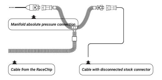
• Disconnect the plug from the manifold absolute pressure sensor.
