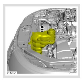
Raise the coolant expansion tank minimum 110mm from its original position.
