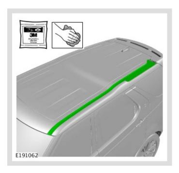
Remove all foam and adhesive tape residue before cleaning the highlighted surface with the provided wipes.
