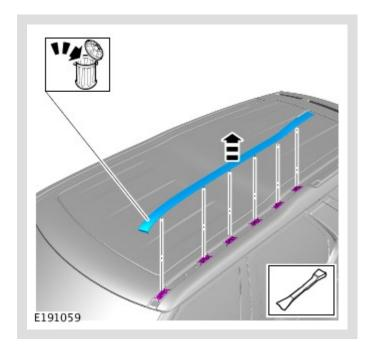
Using a suitable, plastic trim tool, remove Ditch Finisher.
