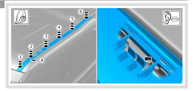
Fit Ditch Finisher making sure locating tabs align with recess in body.
