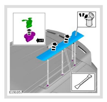
Using a suitable, plastic trim tool, remove trim finisher.
