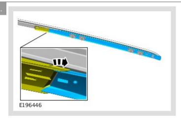
Make sure the tabs of the small highlighted seal are positioned outside of the seal 'O' tabs.
