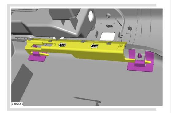
Slide the locking mechanism towards the front of the vehicle until the latches are clear.
