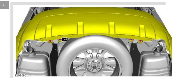
Remove the rear bumper lower fixings.
