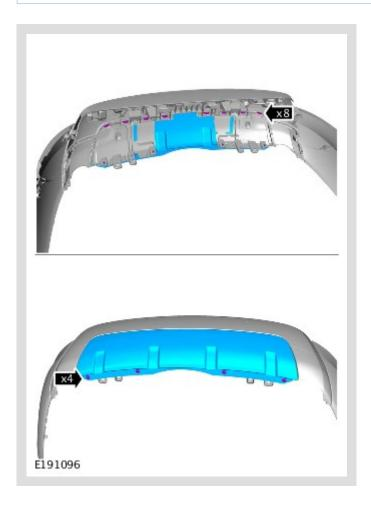
Remove the rear bumper towing eye cover.
