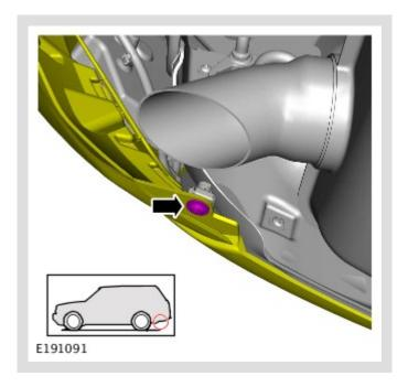
Remove the rear bumper outer fixings.
