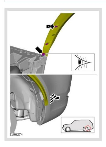
Position the rear wheel arch liner cladding to one side.
