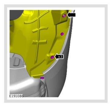
Release the rear section of the wheel arch liner.
