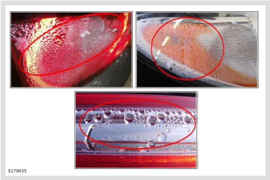
In the photographs shown below, note the drip marks or streaks in the condensation
